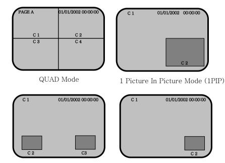
2 Picture In Picture Mode (2PIP) Sequence Picture In Picture Mode
